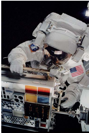
Astronaut installing one the Passive Experiment Containers containing POSS® Nanocomposites onto the International Space Station during STS-105. *Courtesy U.S. Air Force
