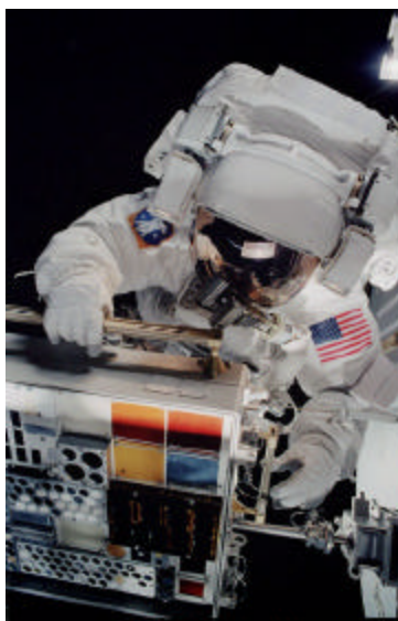
Astronaut installing one the Passive Experiment Containers containing POSS® Nanocomposites onto the International Space Station during STS-105.
