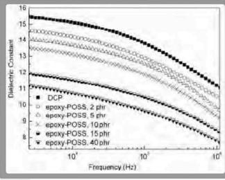
Increasing EP0408 concentration leads to a reduction in the dielectric constant of the rubber
