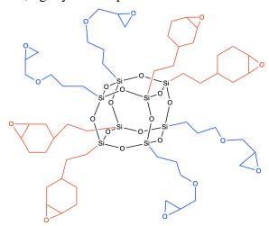
HC0304.11 has found a diversity of uses. It is generally utilized as an additive at 0.5-3 wt% loading levels to impart adhesion and durability in coatings. It is also used as a compatibilizer and carrier of ingredients in coatings and resins. It can also be surfaced glassified under oxygen plasma, corona and UV to provide a tie-layer for coatings or to increase scratch and mar resistance.
