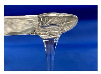
**BENEFITS** UV Cationic and Addition Cure. The combination of reactivity and hydrophobicity provides for interfacial compatibility and dispersion. The high crosslinking capability in combination with i-Octyl provides for resistance to moisture uptake and water repellency, while retaining optical transmission.
